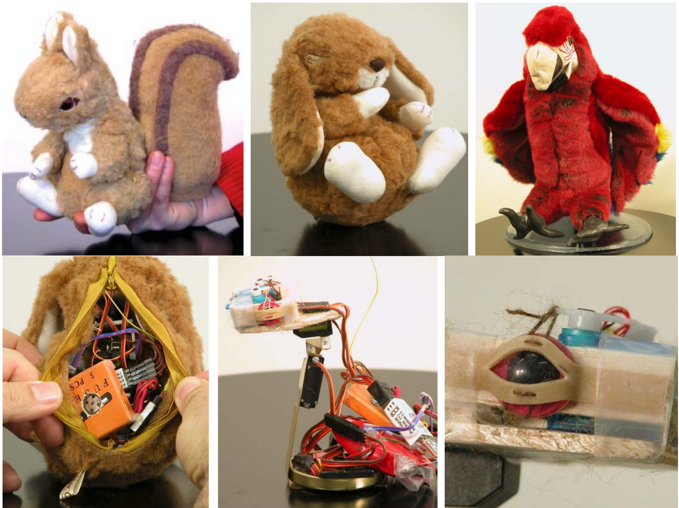
Figure 1: Top row, left to right: squirrel (11cm tall), bunny (10cm tall); parrot (38cm tall). Bottom row: bunny with open back, bunny skeleton, eye and lid mechanics.
