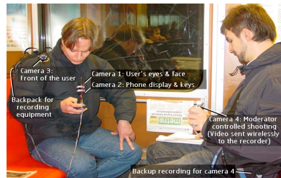
Figure 2. Configuration of recording equipment.
